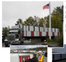
These cruise ship camels feature heavy duty "D" fendering on the vessel side and UHMW wear surface on the Pier side. A unique dock plate system allows seawater to serve as ballast yet freely drain from the camels when not in use. The Camels were so light weight that they required only one truck for shipment.
